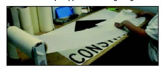
Figure 4.16 Taping of Legend and Transfer Tape to Sign
