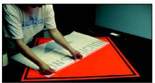
Figure 4.17 **Removal of Backing from Sign Legend**
