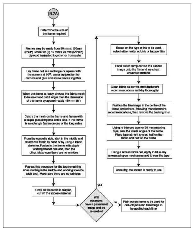
Flowchart B.7A – Construction of a Screen Frame
