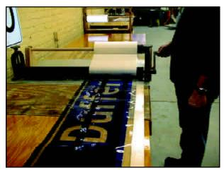
Figure 4.23 – Application of Transfer Tape to Reverse-cut Transparent Sheeting
