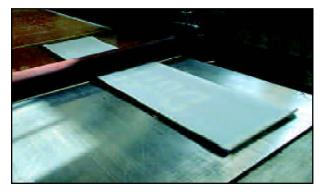
Figure 4.25 – Stripping of Backing from Reverse-cut Transparent Sheeting (first half)
