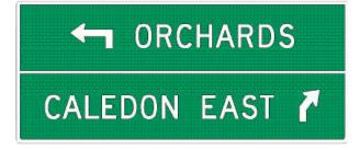
**Location data:** Posted speed is 80 km/h; two-lane rural road (one lane each direction); ground-mounted sign; good vertical and horizontal alignment.
