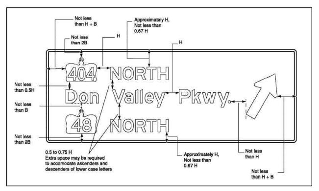
Figure 2.4 – Spacing Guidelines for Text on Directional Guide Signs with Arrows, Crowns & Shields
