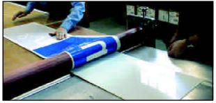
Figure 4.28 – Removal of Transfer Tape
