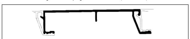
Figure 4.1 – Snap-together Extruded Panel (cross-section)
