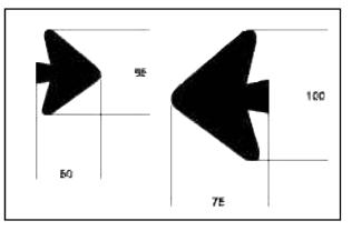
*Placement of Overhead Advance Sign Arrows:* The bottom of the arrow(s) is lined up relative to the bottom of the sign as shown in the Sign Parts Library (dimensions are shown).
